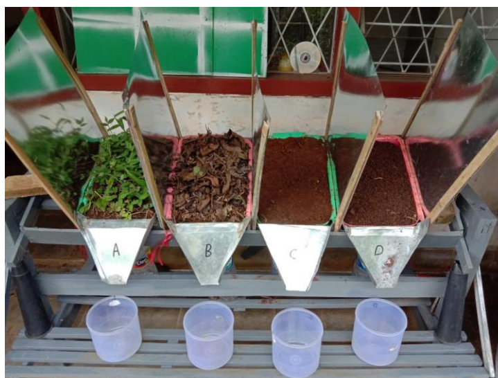
Gambar 1. Rainfall simulator sederhana
